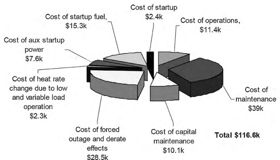
**Figure 3:** Illustrative Shutdown-Start Per Cycle Cost of a 30-Year-Old 500 MW Coal-Fired Steam Plant
