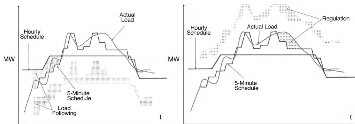
Figure 2: Load Following and Regulation
