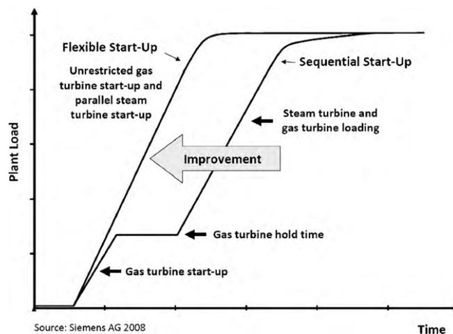
**Figure 4:** More Flexible CCGT Plant Startup Concept
